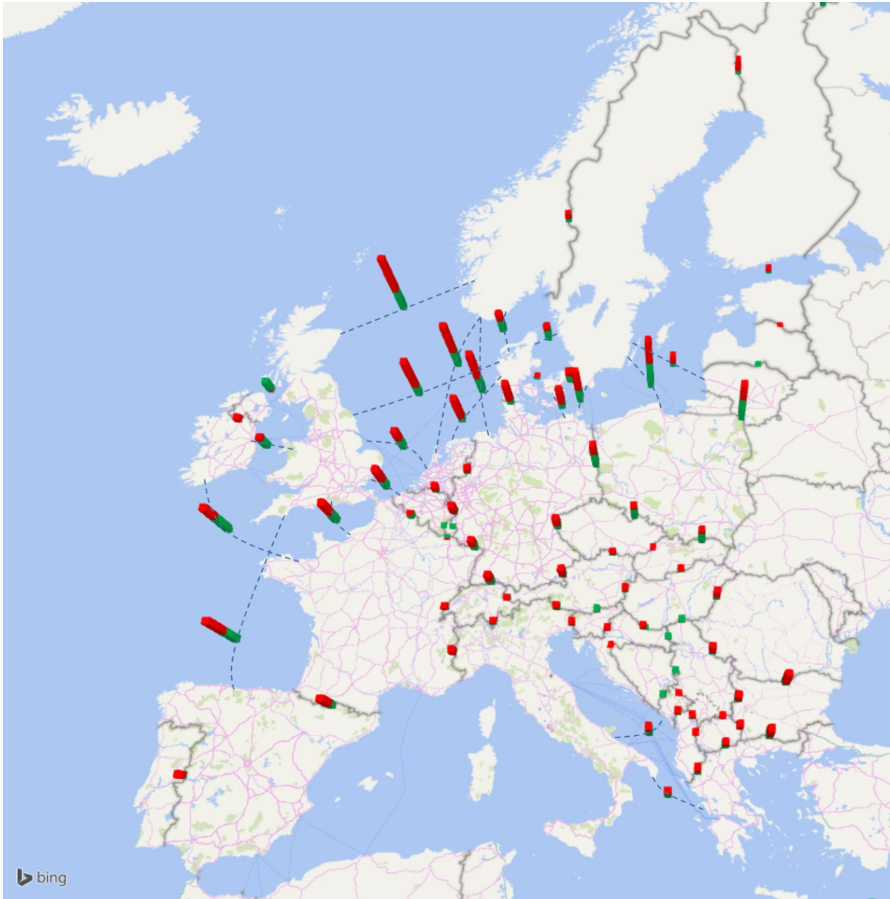
Figure 4 - Reduction in the yearly average of hourly marginal cost spreads in Vision 3, illustrating the benefit of TYNDP investments for European market integration. The total bar height represents the average price spread at each border in Vision 3 without the TYNDP investments; the green bars represent the remaining spread with the market capacity delivered by TYNDP investments.
